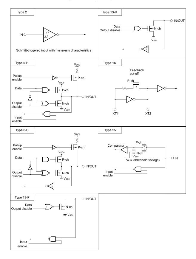
Figure 2-1. Pin Input/Output Circuits
