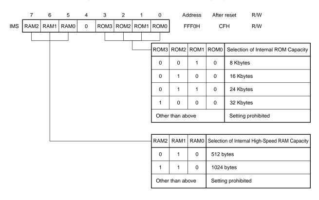
Figure 3-1. Format of Memory Size Switching Register
